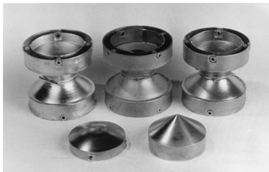
Fig. 4. Three-dimensional ion traps developed in our research laboratory. The upper row (from the left): the axially symmetric ion trap; the axially symmetric ion trap with a cone-shaped endcap electrode (three-dimensional monopole); the ion trap with elliptical electrodes. At the bottom: a hyperbolic electrode and a cone-shaped endcap electrode.
